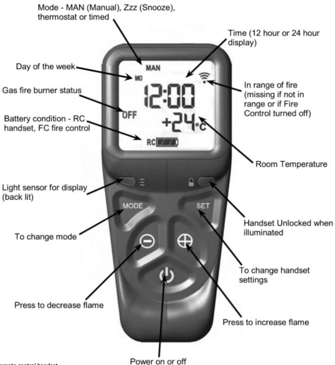
Fig.3 Remote control handset
