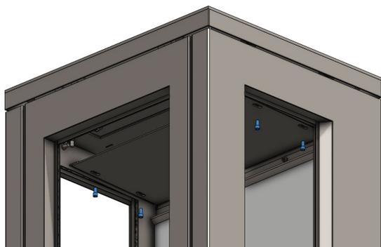
Fig.15 Remove baffle screws
